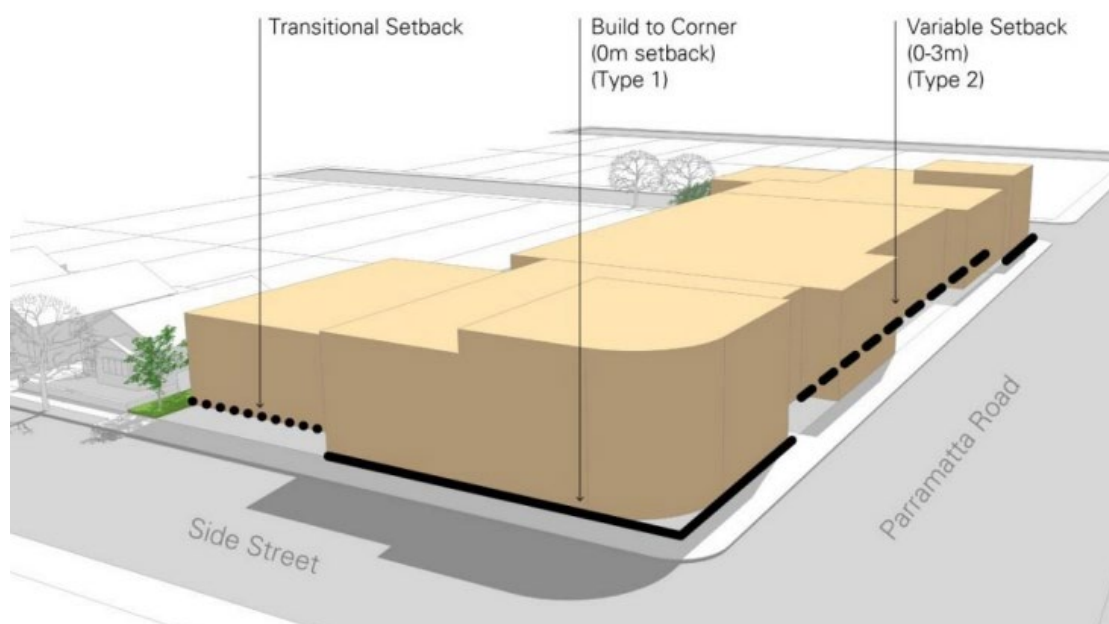
Figure 4: Diagram from the DCP showing the desired envelope and setbacks for corner sites.
